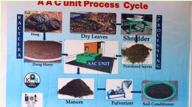
A diagram showing the operation of an Accelerated Anaerobic Composting ACC unit.
