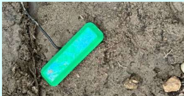
The 3D-printed top of the microbial fuel cell sticking out of the soil. (Northwestern University)
